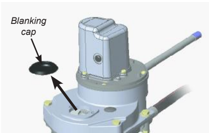
Fig B26 - Installing the rudder feedback unit
